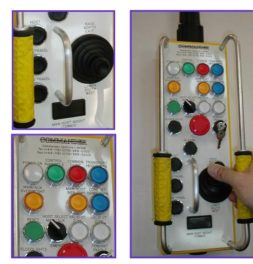
The **COMMANDER<sup>™</sup> BNFL Pattern Pendant Station** has been designed to provide a common style layout which ensures familiarisation by operators if moving from crane to crane. This **COMMANDER<sup>™</sup>** design pendant station also reduces operator fatigue which can be encountered when using outdated mechanically hard 'Euclid style' 3 step push button mechanism used on older cranes.
